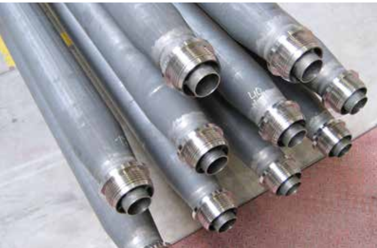
Steam reformer pipes
