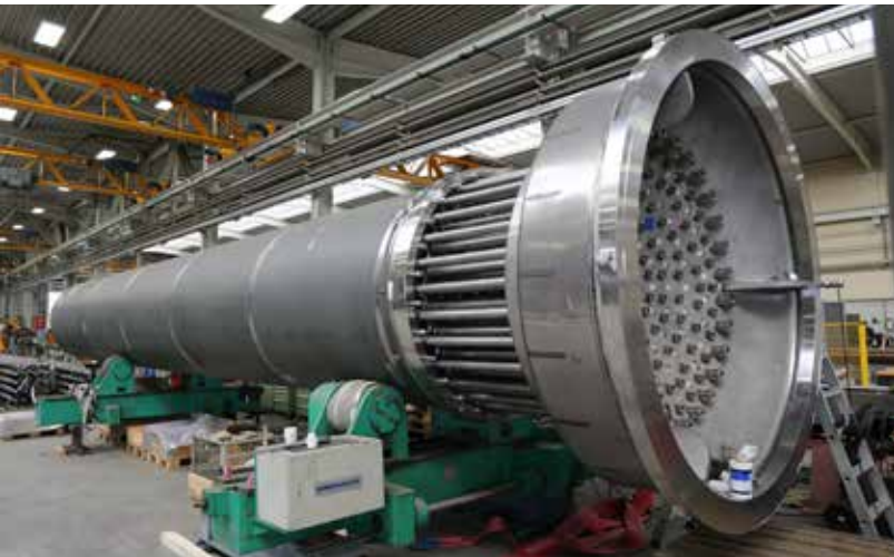
Heat exchange reformer
